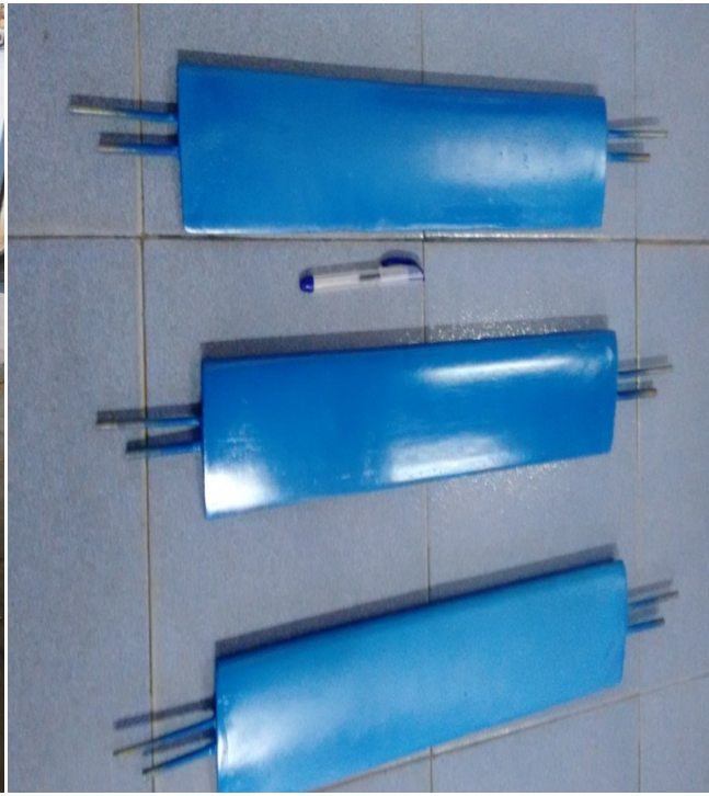
Flow Modifier, Dept of Mechanical Engineering. Non standard acrylic and FRP blades.
