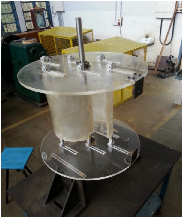
Flow Modifier, Dept of Mechanical Engineering. Non standard acrylic and FRP blades.
