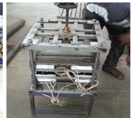
Heater assembly under construction
